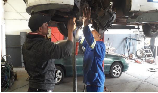
Removing a gearbox for repairs
