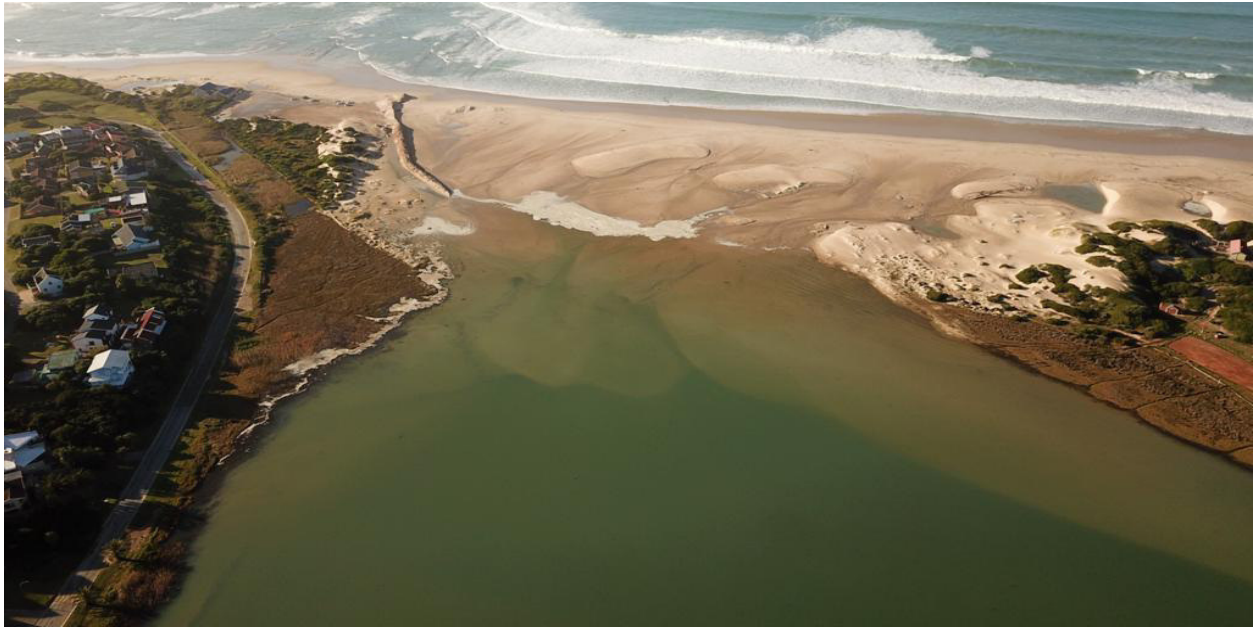
Fig. 15. Photo of the estuary mouth on the 4 th July 2020. Overtopping of the berm occurred across a wide area leading to the rise in water level in the estuary. (photo provided by Councillor Brenton Williams). Note the sand delta in the estuary formed by overtopping events.
