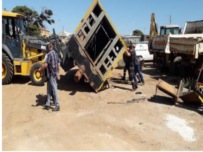
Old sanitation unit removed from burned-out truck and refitted to refurbished chassis cab.
