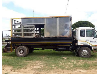
Old sanitation unit removed from burned-out truck and refitted to refurbished chassis cab.
