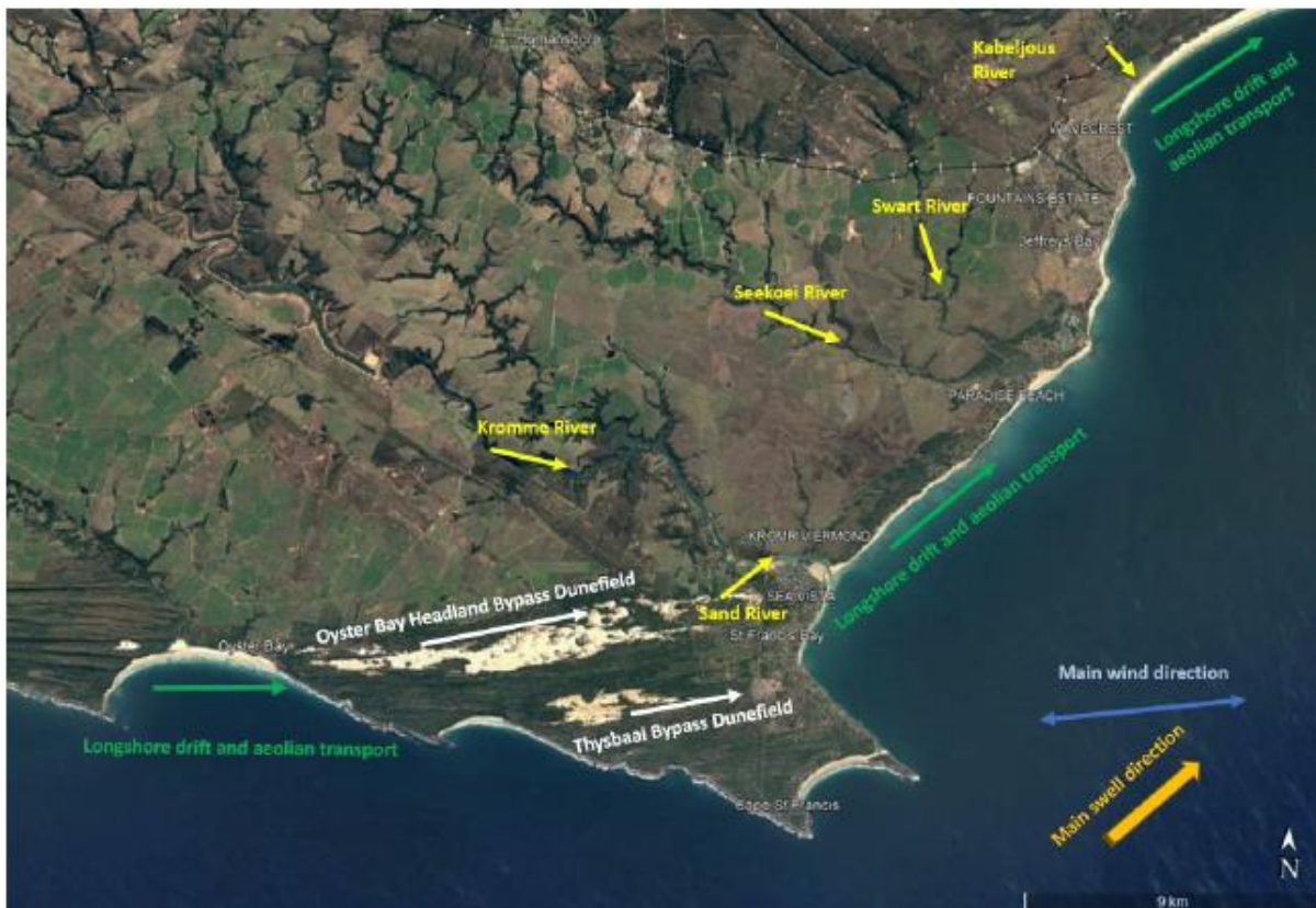
Figure 4.15: The main sediment pathways of the KLM coastal zone (van der Waal, 2024).
