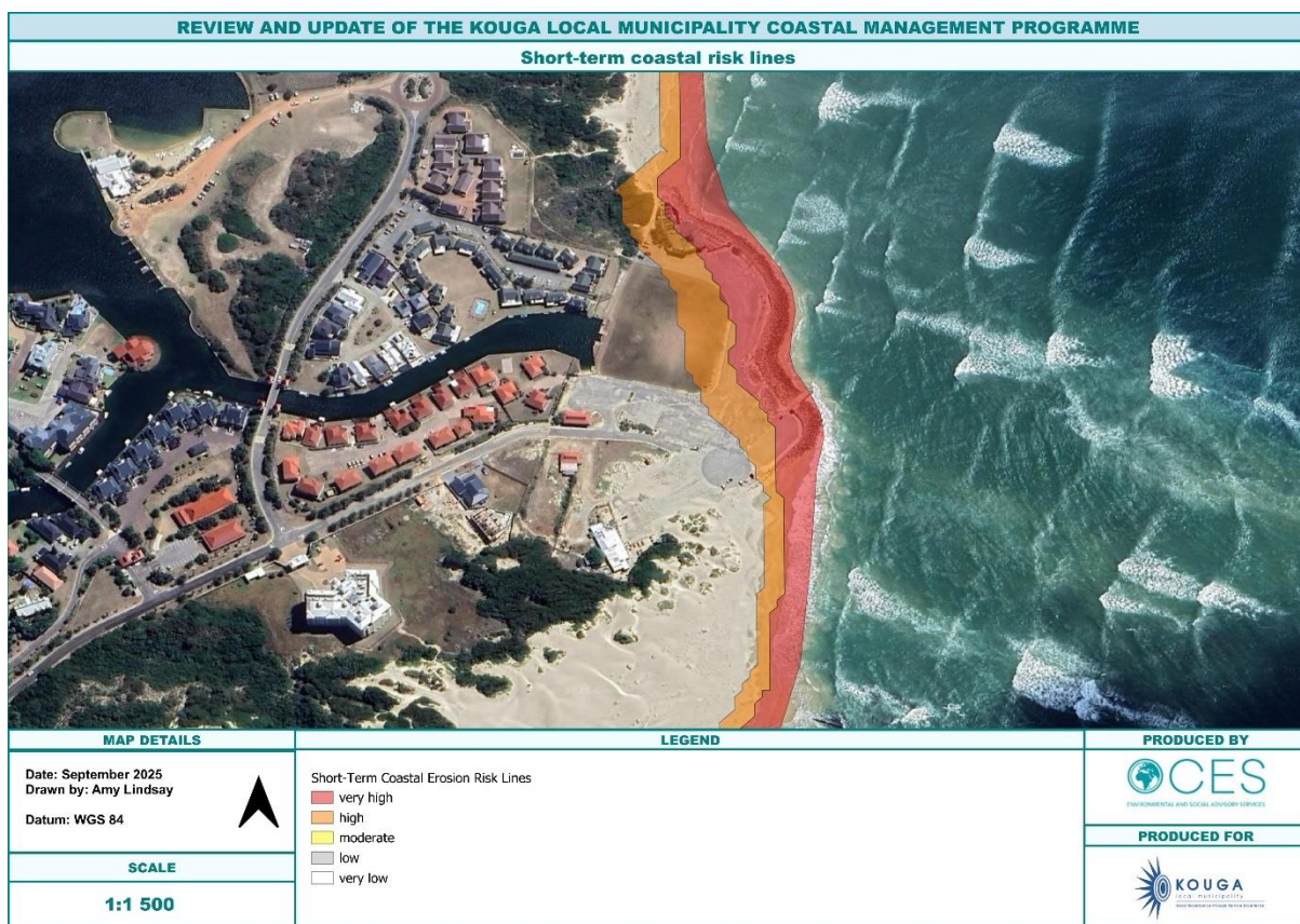
Figure 4.19: Short-term coastal erosion risk lines along a section of Marina Martinique.
