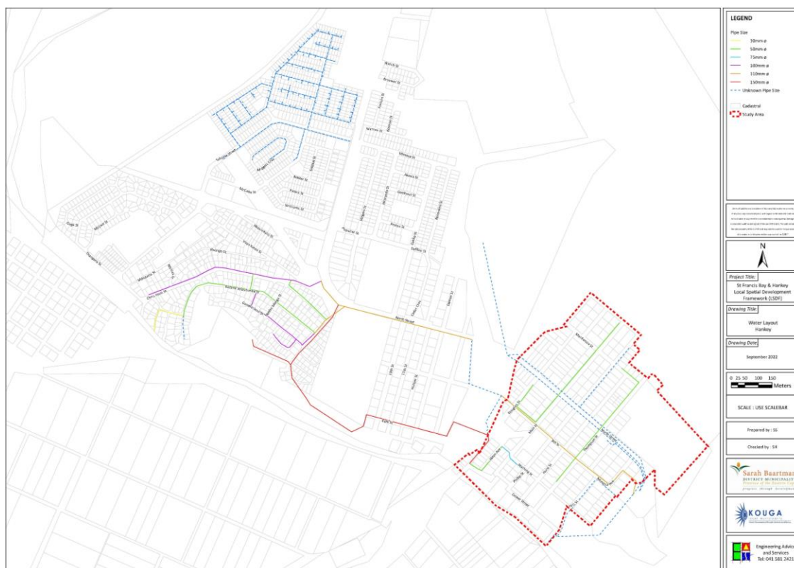
Existing Water Reticulation Network (Hankey)
