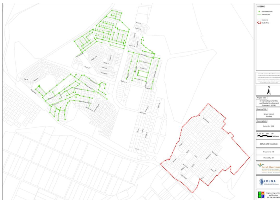
Existing Sewer Reticulation Network (Hankey)
