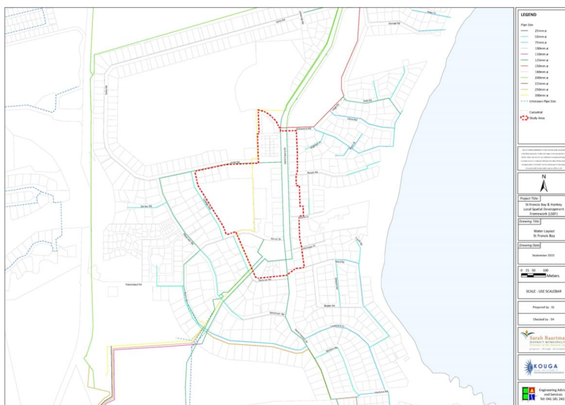
Existing Water Reticulation Network (St Francis Bay)
