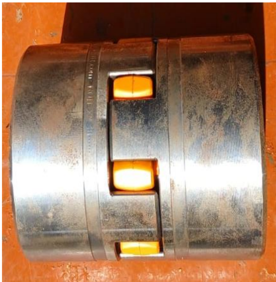
13 Spider gear plus rubber damper
