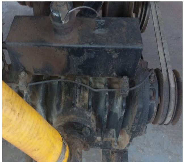
20 Vacuum exhauster pump "left turn"
