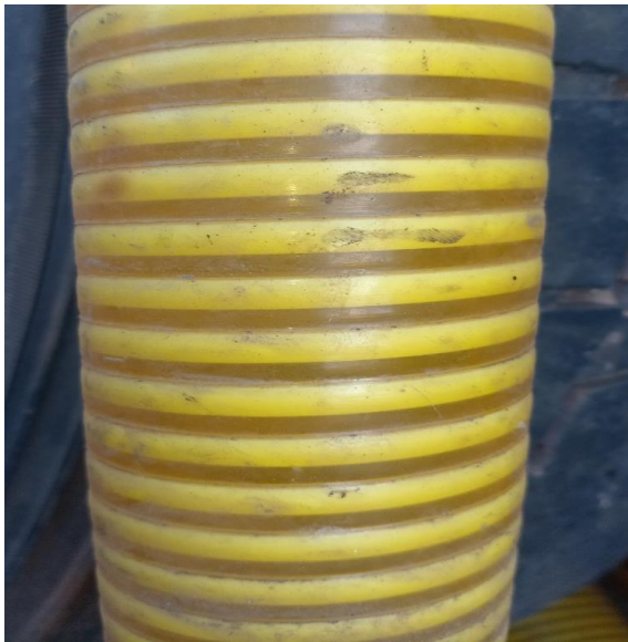
17 Kanaflex hose 120mm outside diameter
