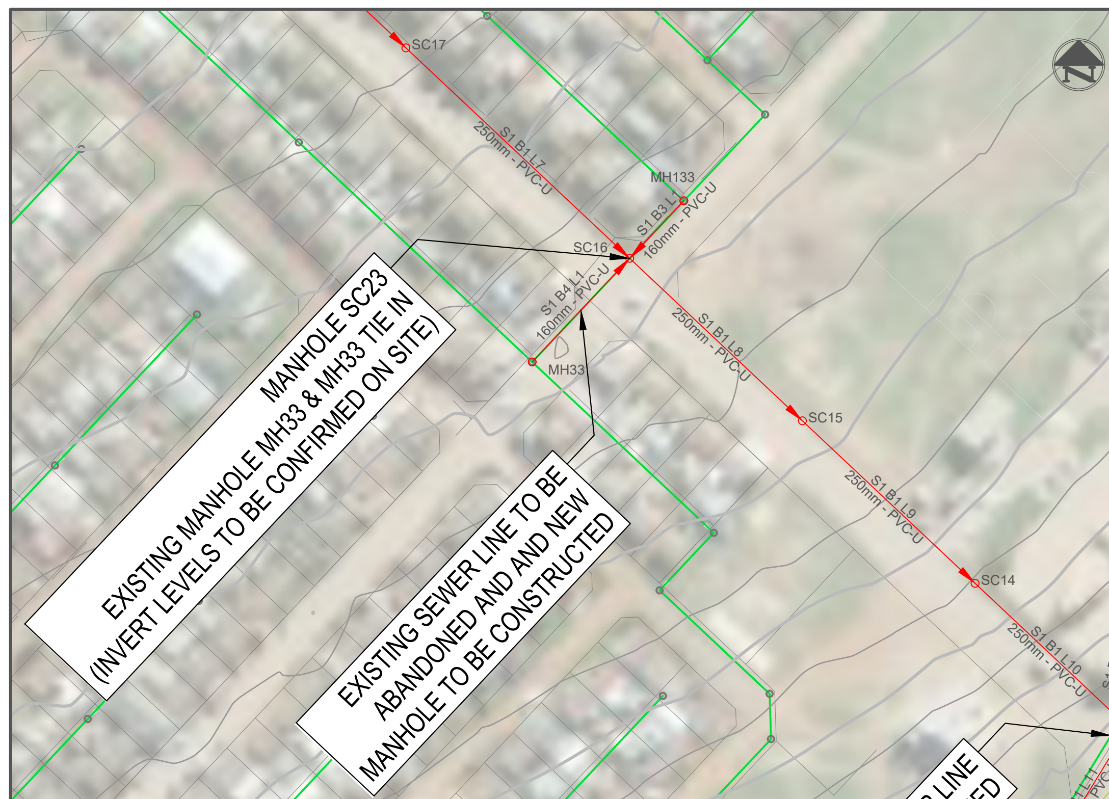
LAYOUT PLAN: MANHOLE SC17 TO 14 SCALE 1:1000
